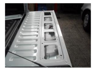
2) Undo 2 Bolts from the Handle (this is the location you will mount the power lock)
