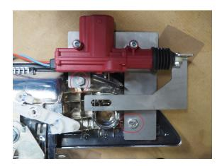
5) Refit Key Barrel—Simply slide back into position, Ensure you slide through power lock and onto the trucks lock mechanism
