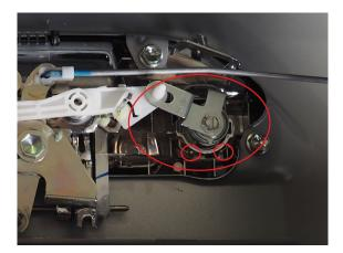
4) Mount Power Lock—Fix into position by reusing the bolts you removed in step 2
