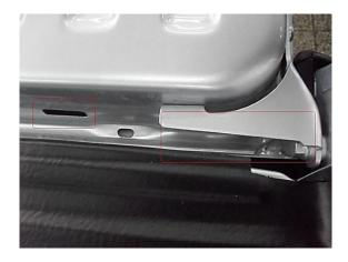
8) Pull up Door sill guard to locate vehicle wiring loom and allow access to the Power lock cable
