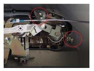
3) Remove Key barrel lock (press the spring clip together and simply pull out)
